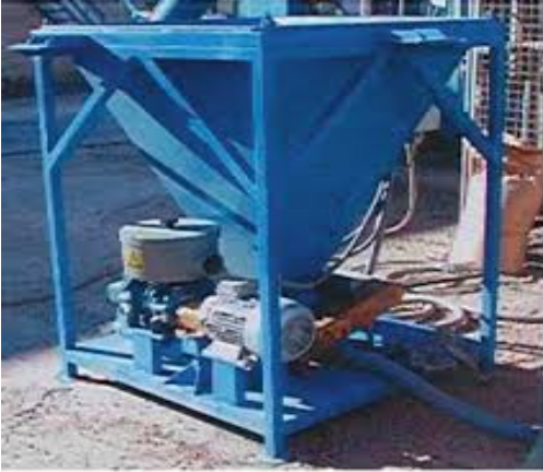
Example of Pneumatic Dosing System
