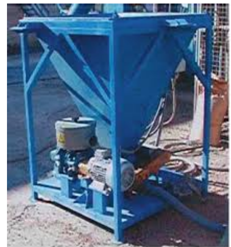
Pneumatic dosing plant
